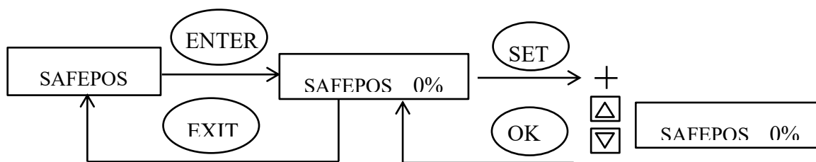
Figure 29. Operating structure SAFEPOS
